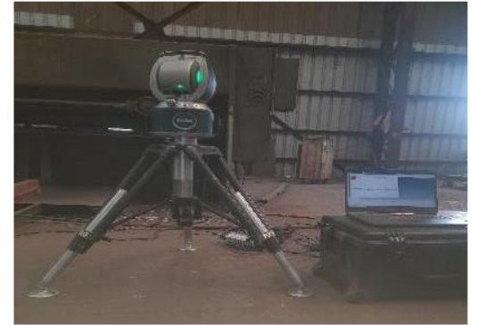
Laser tracker measuring device (Faro vantage)
