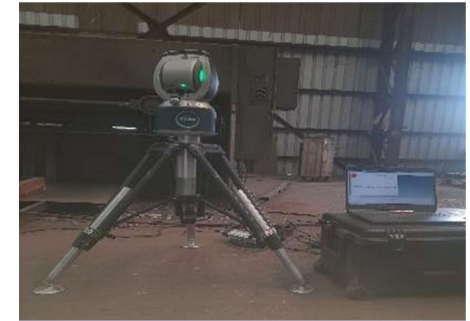
Laser tracker measuring device (Faro vantage)
